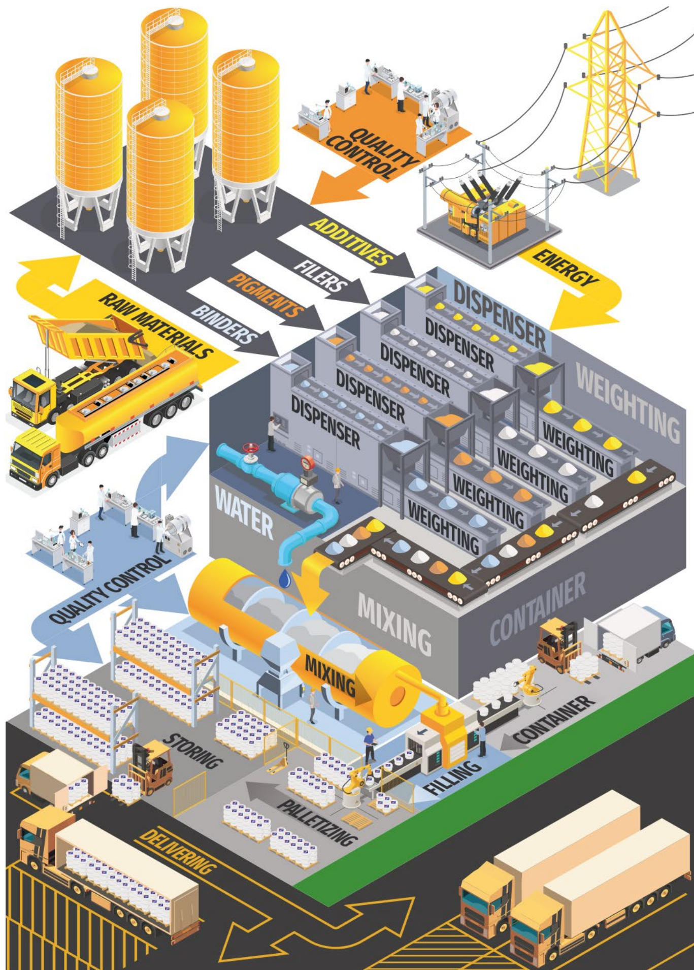
Figure 4. Production process – paints and primers (scheme)
