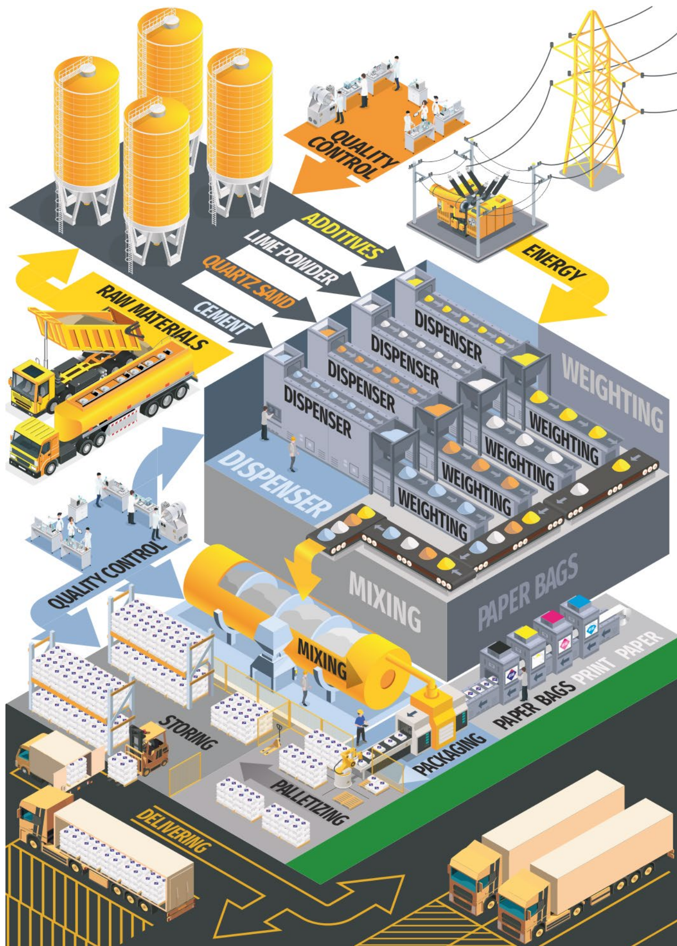
Figure 2. Production process – dry mixes (scheme)
