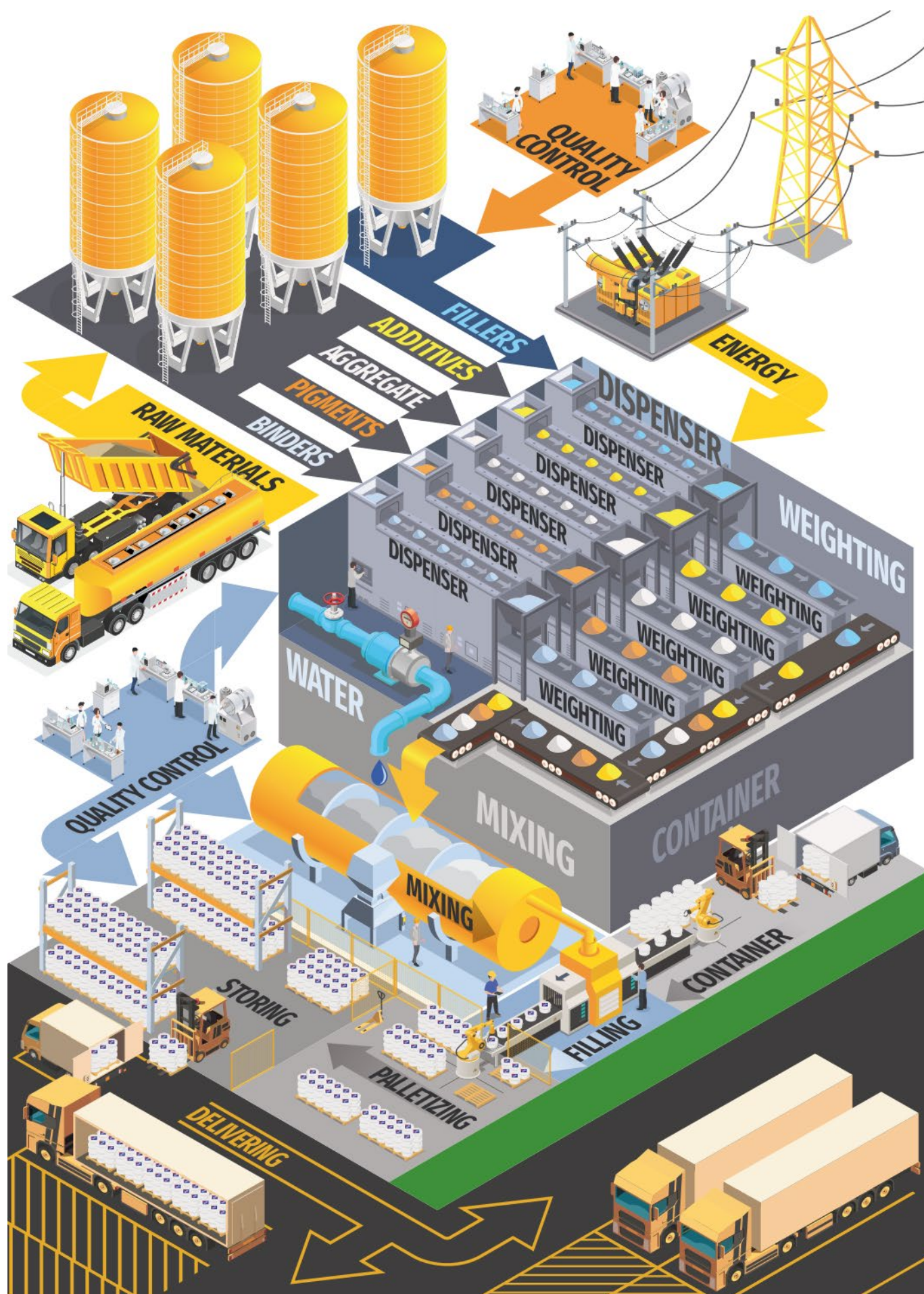
Figure 3. Production process – ready-to-use renders (scheme)
