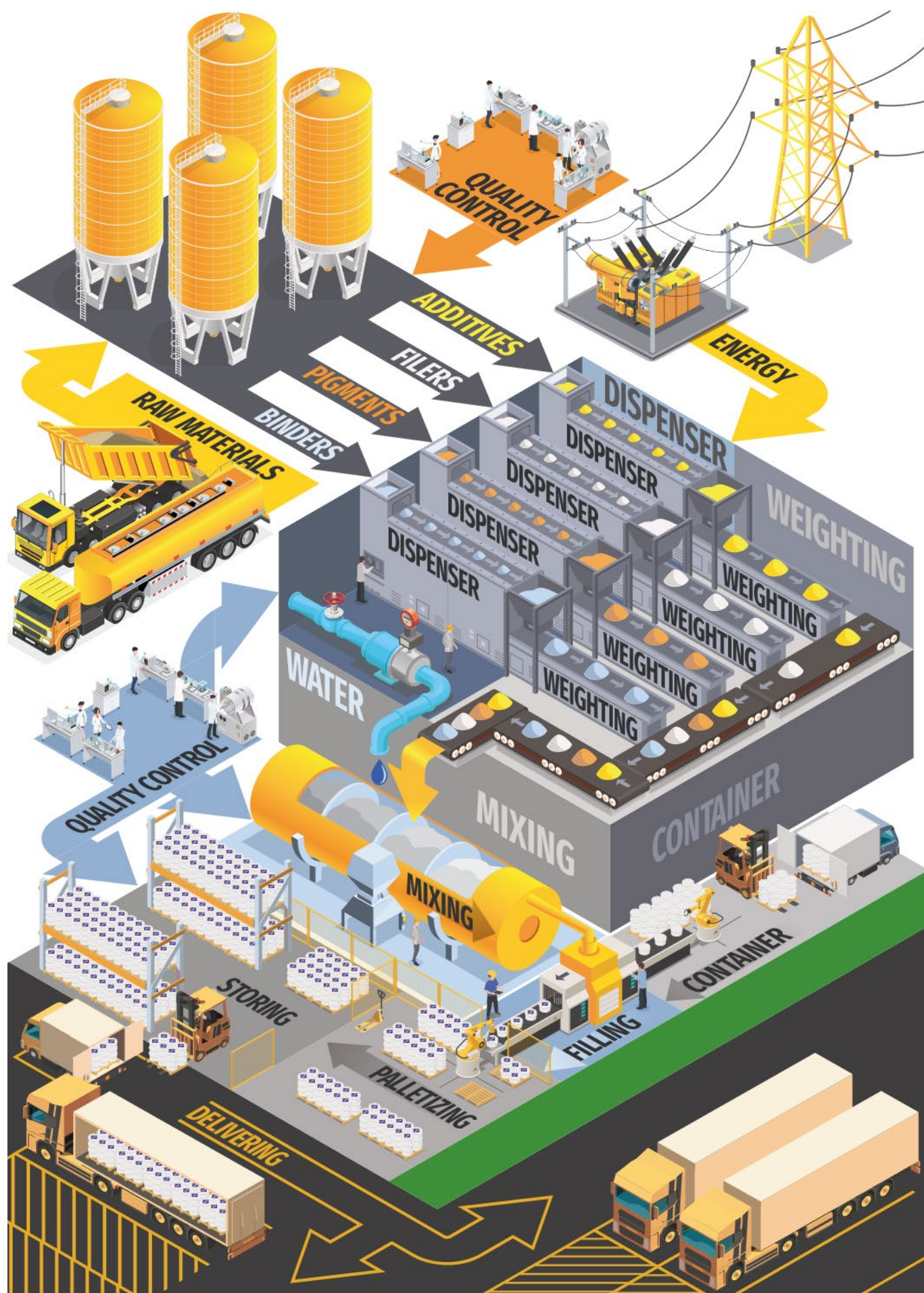
Figure 4. Production process – paints and primers (scheme)
